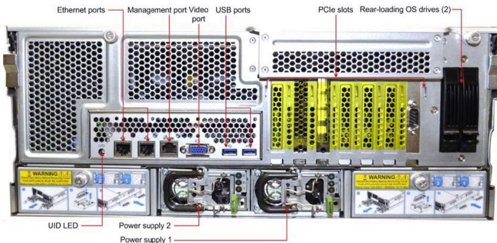
Figure 1. Rear of appliance with card slot highlighted
