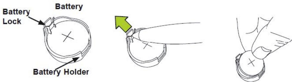
Figure 17. Remove the battery
