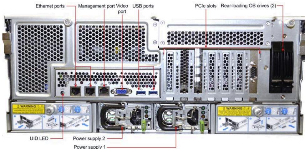
Figure 10. Rear panel I/O ports for the appliance
