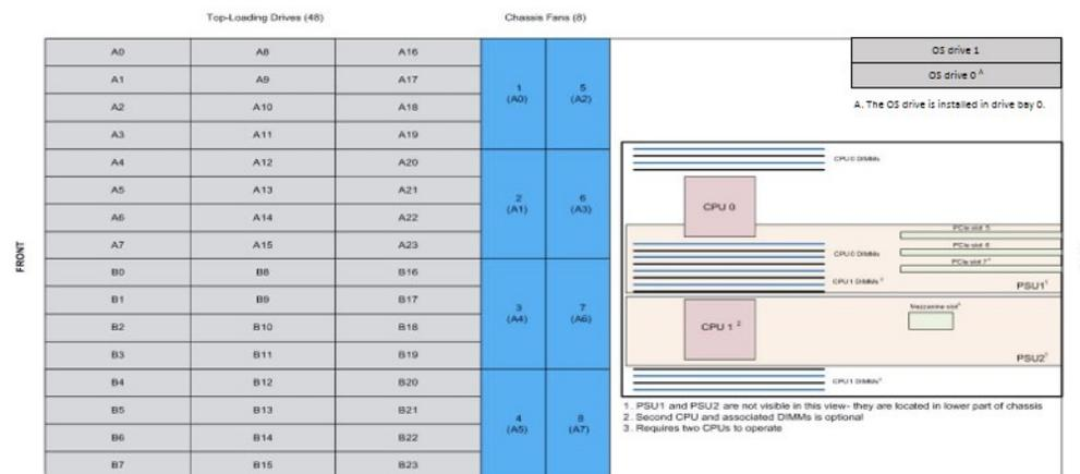
Figure 11. System diagram
