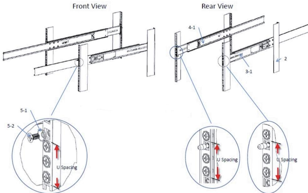
Figure 6. Attach the rack rails to the rack
