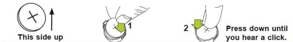
Figure 18. Install the battery
