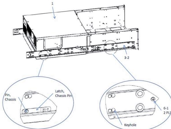
Figure 5. Install the chassis slide rails to the appliance
